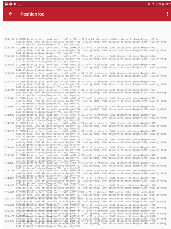
Figure 23: Decawave DRTLs Manager Position Log
