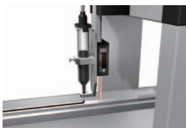
Controlling the height of a dispenser nozzle
