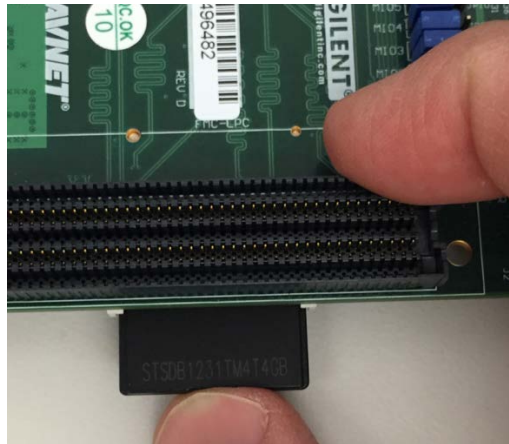
Figure 3. Inserting the SD card into the ZedBoard.
